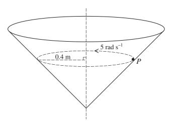
A particle *P* of mass 0.5 kg moves in a horizontal circle on the smooth inner surface of a hollow cone which is fixed with its axis vertical and its vertex downwards. *P* moves with angular speed  $5 \text{ rad s}^{-1}$  in a circle of radius 0.4 m (see diagram). Show that the semi-vertical angle of the cone is  $45^{\circ}$  and calculate the magnitude of the force exerted on *P* by the surface of the cone. [6]
